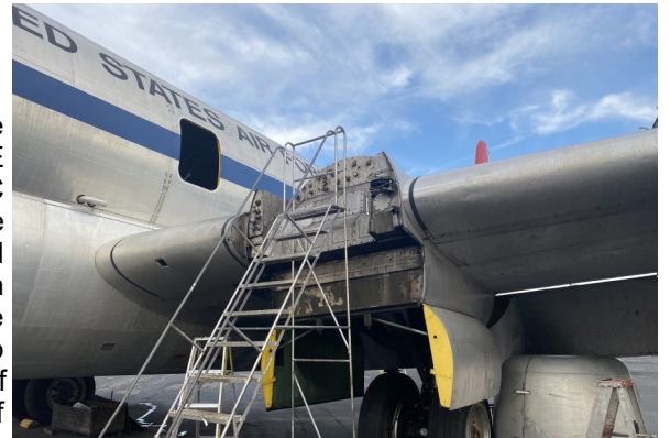
THE #2 POSITION OF C-97G "ANGEL OF DELIVERANCE" AWAITS A REPLACEMENT R4360-59B.
