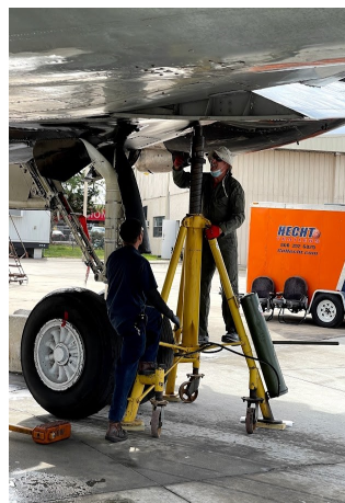
JASON PENCE AND DAVID COBAUGH SETTING A JACK IN PLACE UNDER THE WING OF THE C-54.
